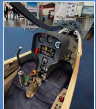
A one-piece instrument panel, battery modules and fairing for the wingtip wheels were created with 3D-printed parts
