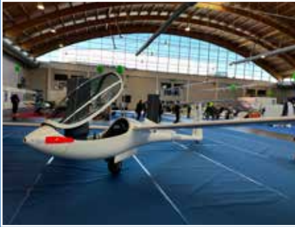
The E-ROP features a 1.2-metre front electric sustainer (FES) developed by LZ Design
